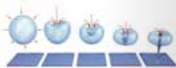
COLLAPSE OF A CAVITATION BUBBLE (SCHEMATIC) CLOSE TO AN ACOUSTIC INTERFACE (STONE SURFACE) | Fig. 19
